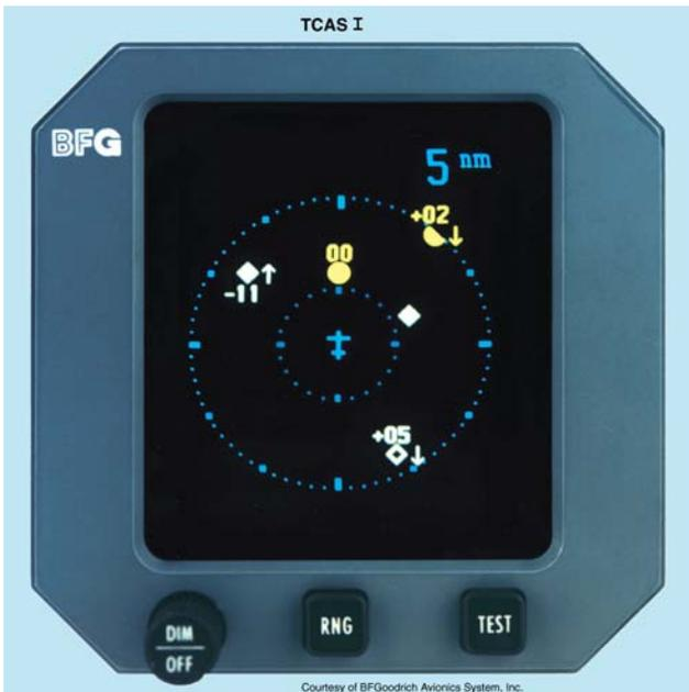
Figure 1-13. Traffic Alert and Collision Avoidance System.
